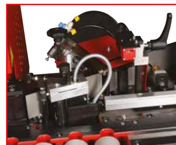
Stanz- und Leimaggregat punching and glueing device
